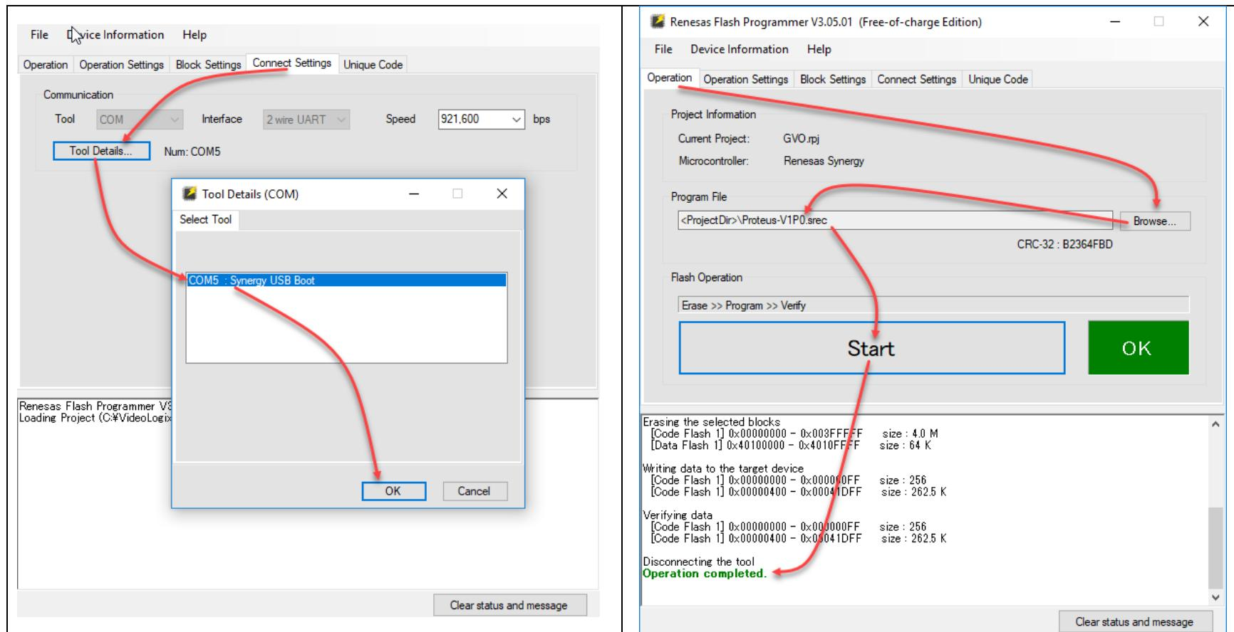
7. After 'Operation completed', Toggle CFG switch in the rear panel to the upper position
